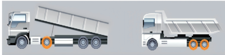
Recommended wheel position: Drive wheel position
